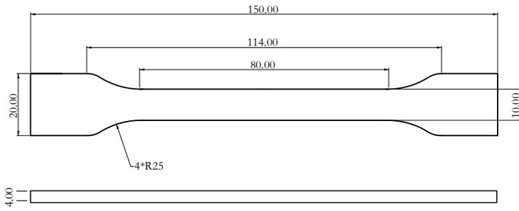
Tensile testing specimen; ASTM D638 (ISO 527, GB/T 1040)
