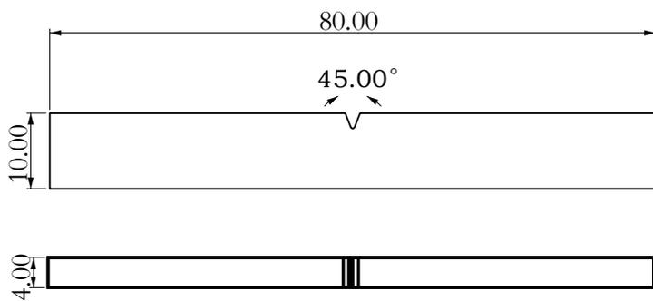
Impact testing specimen; ASTM D256 (ISO 179, GB/T 1043)
