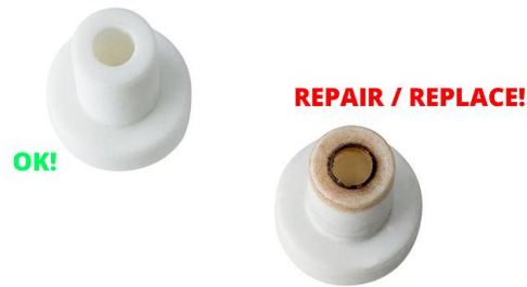
Check your PTFE (if your printer has this in the hotend) for problems. (Brown / Crunchy = bad)
