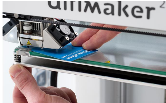
Prepare your plate for the perfect 1st layer / following your 3D printers bed calibration method (make sure to do it properly and maybe even 2 times)
