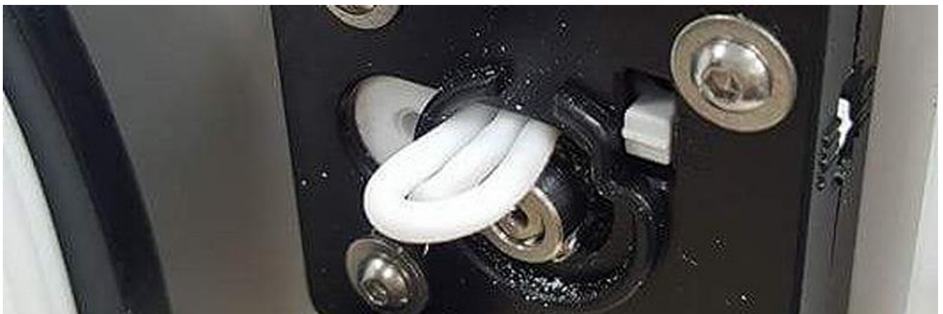
A surprising example of what can go wrong when you don't have the right feeder for printing flexible filament.
